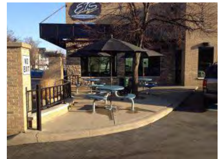
The above represents seating that is removed from the parking facility by a minimum 6" elevation, but lacks the necessary railing.
