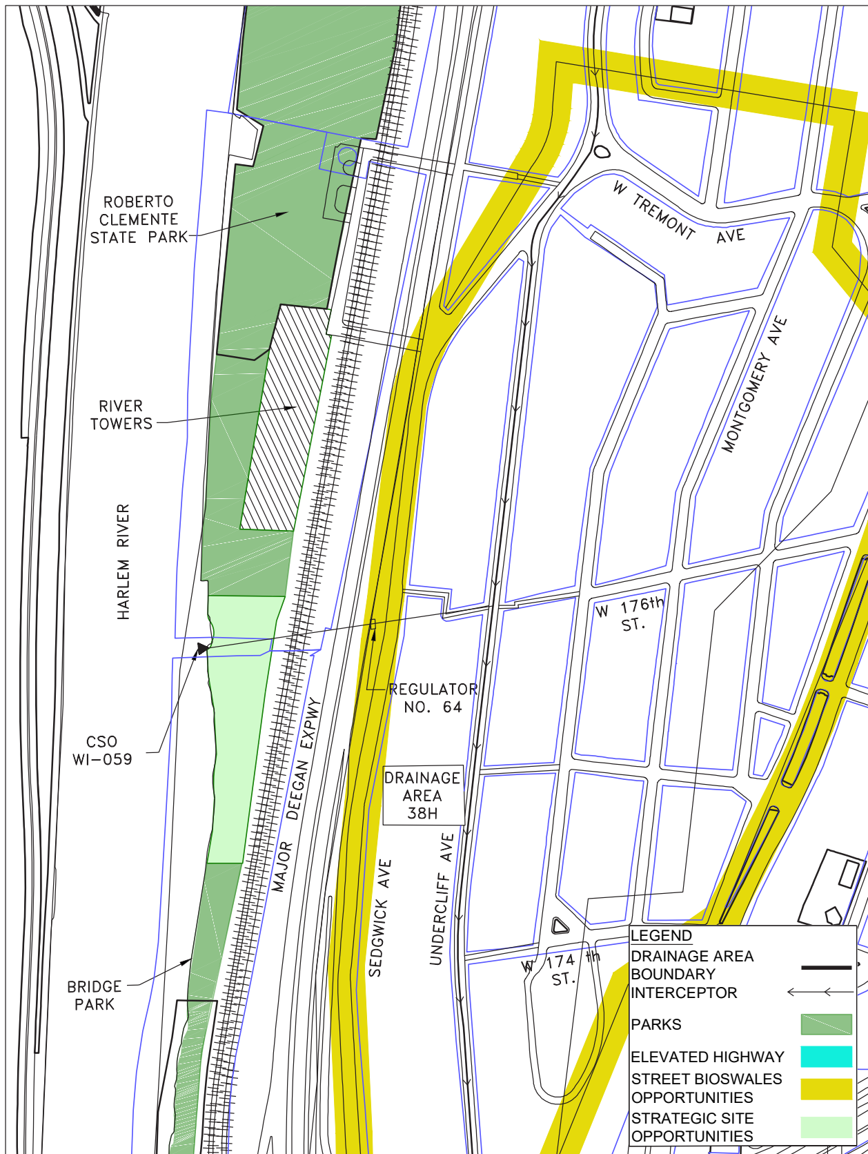
Figure 29. Infrastructure and Drainage Map 4: Bridge Park to RCSP Area (Source: STV, utilizing DEP drainage maps)
