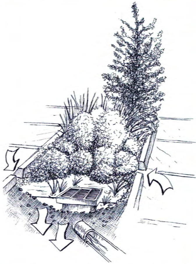
Site 12, 16, & 18: Parking Lot Island Raingarden: curb cut or wheel stop openings into shallow depression with raised outlet pipe for storage.
